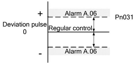
When Pn047 is set to 1, if the range of error counter overflow(Pn031) is set too small, alarm A.06 may occur when running at high speed.
