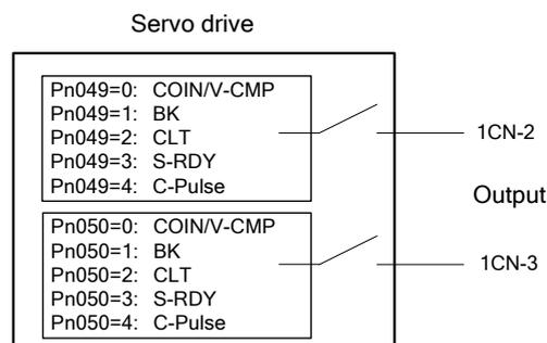
The following table shows the pin number definition for Pn049 (correspond to pin 1CN-2 output), Pn050 (correspond to pin 1CN-3 output).
