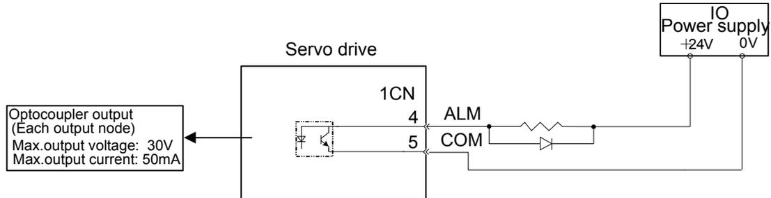
External +24V I/O power supply is required, since there is no +24V power supply available inside servo drive.
