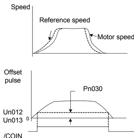
Un012:error pulse counter low position monitoring
