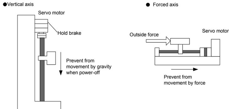
Make sure servomotor is mechanically separated before confirming action of servomotor and brake active (holding brake). If all the parts are moving well, connect servo motor to the machine.
