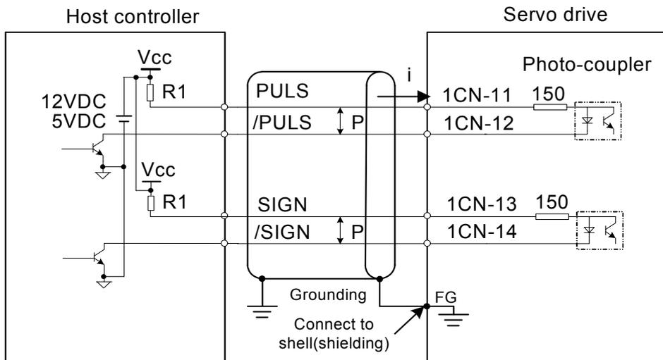
The right current limiting resistor R1 should be used according to current requirements ( $i = 10\sim 15\text{mA}$ ) :
