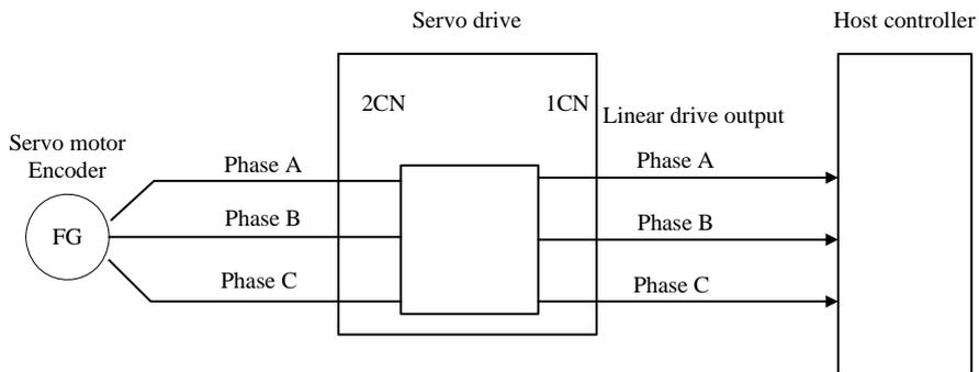
Output circuit is bus drive output. Make circuit connection with reference to following circuit.
