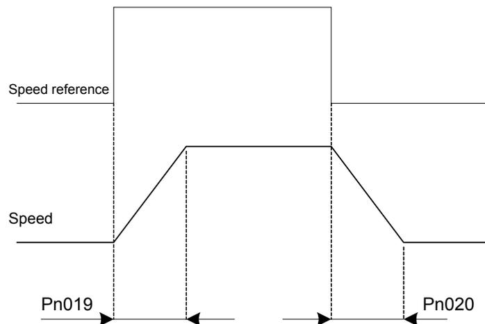
Pn019 and Pn020 are linear acceleration/deceleration time. In the event of rather large jolt which may occur because linear acceleration/deceleration time are applied, Pn021 can be selected and set to smooth running.
