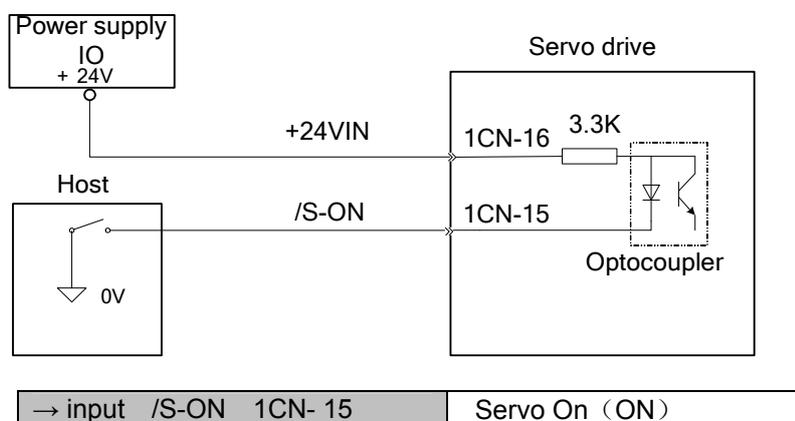
Switch servomotor between Power on and Power of, when low level is active.
