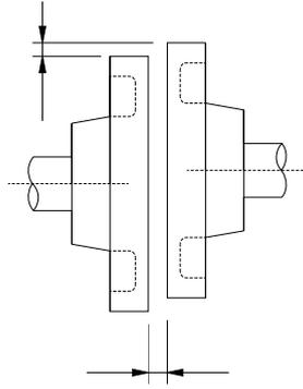
Measure this at four quarter positions of a cycle. The difference between the maximum and minimum measured value must be less than 0.03mm. (Rotate together with shaft connectors)
