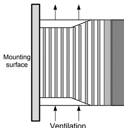
A cooling fan can be mounted for forced-air cooling of the servo drive at request.
