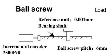
$$\text{Load movement amount of bearing shaft one round rotation} = \frac{6\text{mm}}{0.001\text{mm}} = 6000$$
