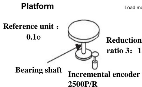
$$\text{Load movement amount of bearing shaft one round rotaion} = \frac{360^\circ}{0.1^\circ} = 3600$$
