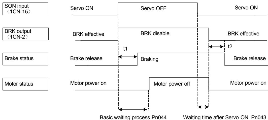
t1,t2:determined by external relay and brake loop move time
