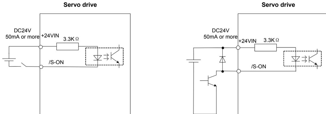
If the relay contact input is used, the relay must be suitable for low electric current, otherwise it causes signal receiving faults.
