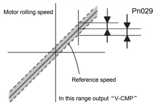
With the user's constant as below, the range of output /V-CMP can be designated.
