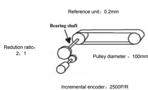
$$\text{Load movement amount of bearing shaft 's one round rotation} = \frac{3.14 \times 100\text{mm}}{0.2\text{mm}} = 15700$$
