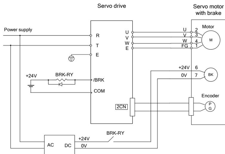
BRK-RY: brake sticking control relay
